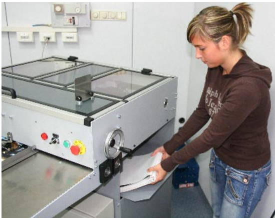
After feeding all pages, the prepared staple of pages can be removed from the collection area.
