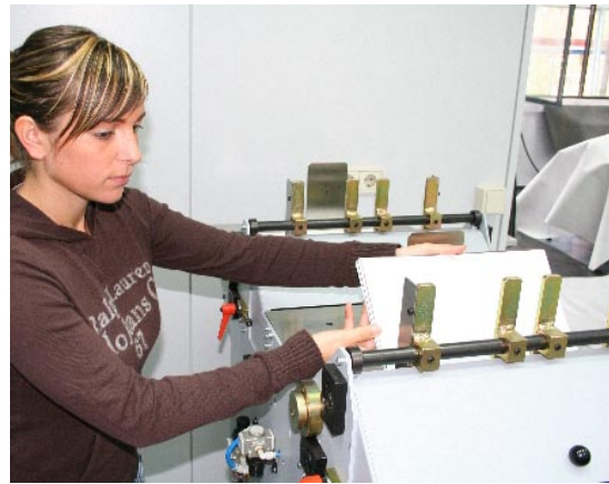
The Auto-Feeder is equipped with the creased/ folded pages and suitable card boards. (card boards must be cut to match the pages size)
