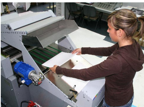
The creased/folded pages and card boards are carried via an automatic transport system to the gluing machine whereby on the lower page side glue is automatically applied. After this, the material is transported via a transport belt to the mounting station.
