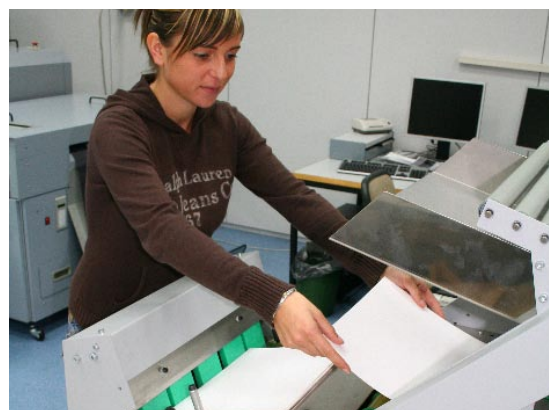
The pages and card boards (with a thin glue film applied at the lower side) will be mounted to a book block. And then pressed in a suitable book press for min. 10 hours (ideally over night) to dry sufficiently. After drying, the book block is cut and mounted into a suitable book cover.
