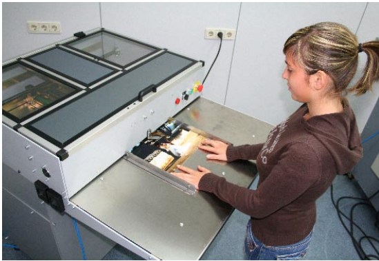
Double sided album pages are fed via adjustable guides into the automatic creasing/folding machine.
